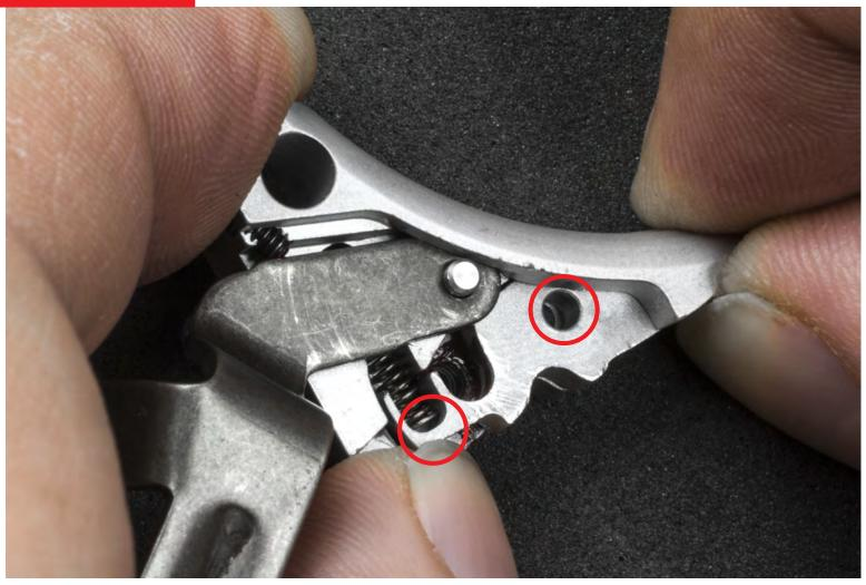
Align the safety lever to capture the safety lever spring and align the pivot hole with the hole in the trigger shoe.
