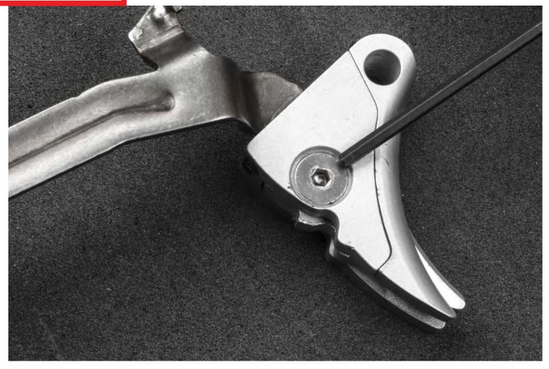
Install the side plate screw with the included wrench and snug the screw. **DO NOT OVERTIGHTEN.** Loctite<sup>®</sup> 222MS (purple) thread locker may be used to prevent screw loosening.
