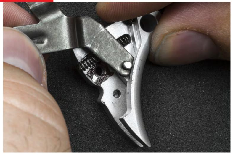
Insert the pin through the trigger bar and into the trigger shoe. If needed, use pliers to help seat the pin.
