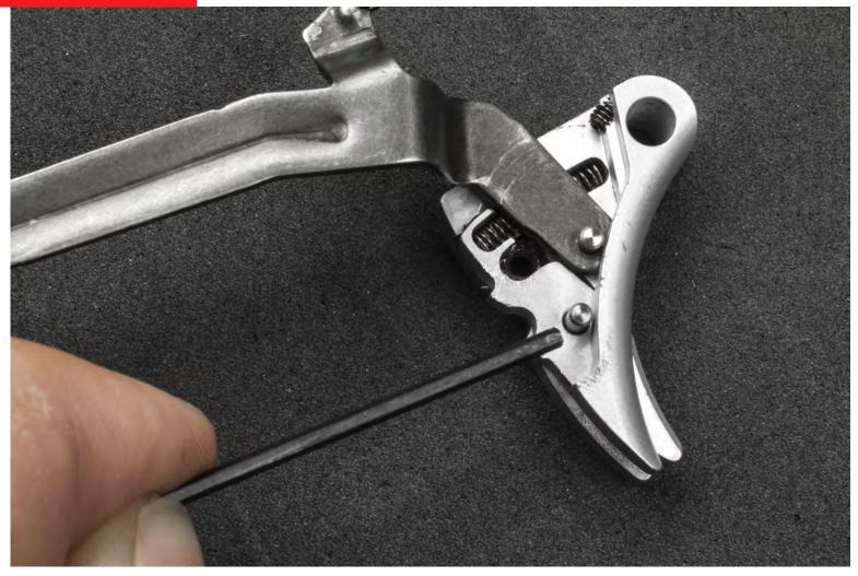
Insert the pin through the safety lever and into the trigger shoe. If needed, use pliers to help seat the pin.
