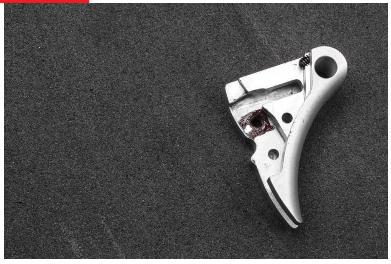
Lay the trigger shoe on a flat surface as shown.
