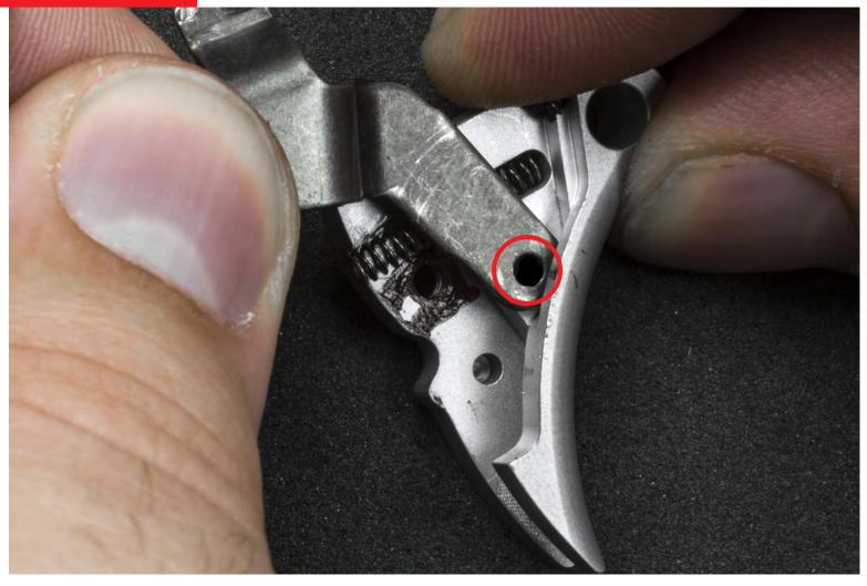
Align the trigger bar over the safety lever spring and align the trigger bar hole with the hole in the trigger shoe.
