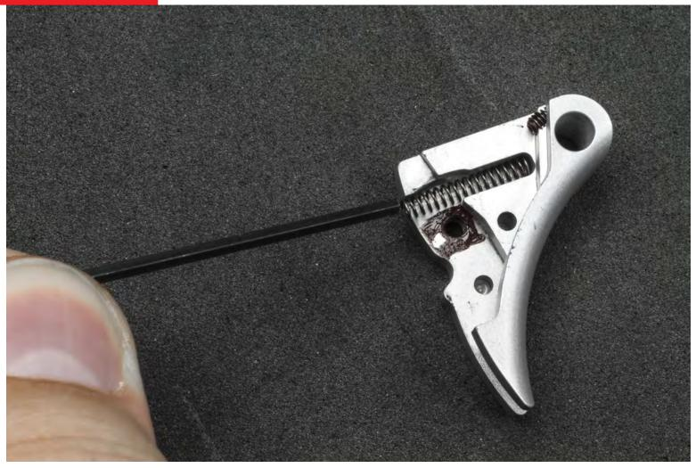
Insert the safety lever spring into the slot as shown.
